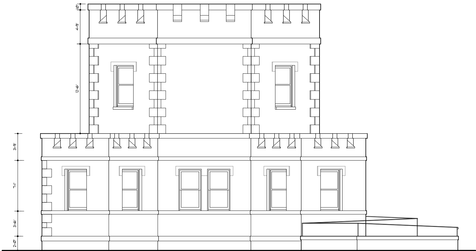
1 EXISTING WEST (CAMPUS) ELEVATION EA202 SCALE: 1/4" = 1'-0"
